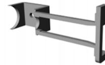
Before securing the cylinders to the brackets, insert a 16BA screw as shown. If using epoxy to assemble filling the cavity between the cylinder and bracket with epoxy will secure the screw otherwise solder the head.
